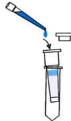
Figure 6: Pipetting of the extract onto the spin column
